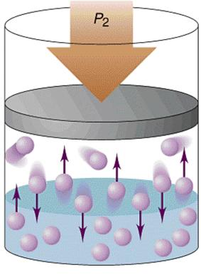
The amount of gas that will dissolve in a liquid is proportional to the partial pressure of the gas in contact with the liquid.
